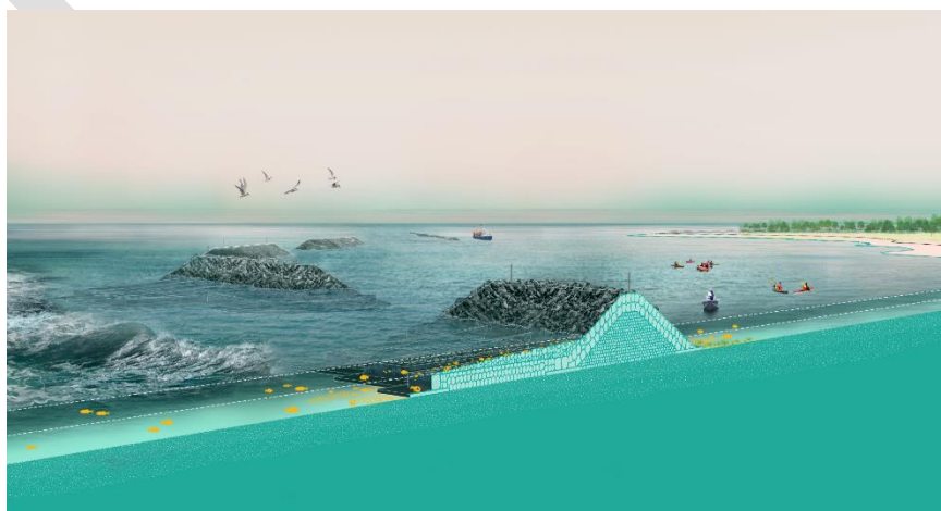
Figure 71. Conceptual rendering of the living breakwaters project off Staten Island (Source: https://stormrecovery.ny.gov/learn-more-about-living-breakwaters-project )
