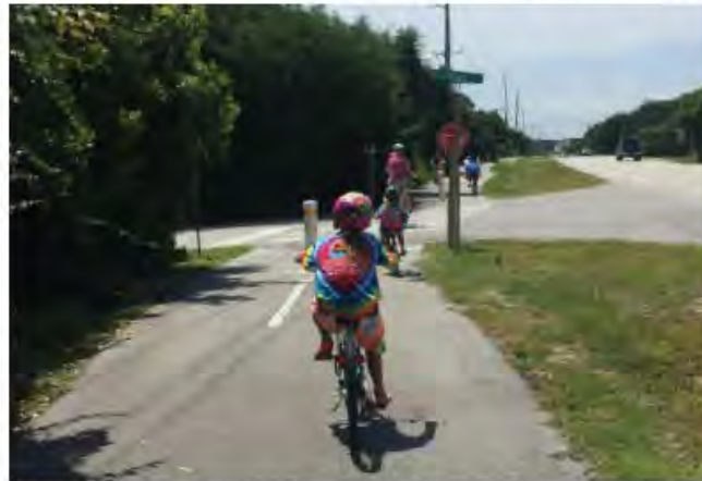
Example of a separated greenway along two-lane highway with a grass swale to increase safety.
