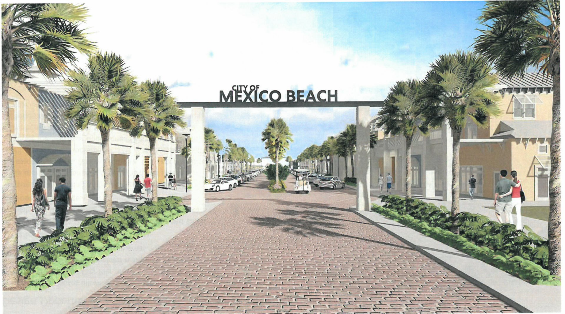
Illustration of entry to 37th Street and mixed use development. Sustainability features include planted swales to capture runoff and pervious pavers to increase infiltration.
